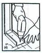
Fasten framing to structural column on center-line and plumb.
