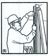
Locate and scribe center-line of structural column. Cut and instal studs to structural column.
