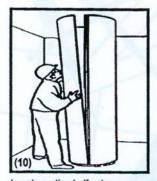
Locate mating half column cover and position around skeleton against vertical stud. Shim at base to match first column cover half.
