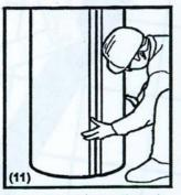
Insure fit and fasten through column and into stud on 16" centers. Tape and float joints.
