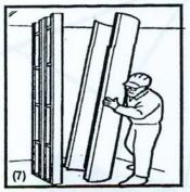
Locate first column cover half and position over scribed circular line on floor. Shim at floor if necessary.
