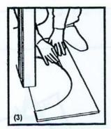
Prepare a template with a cutout representing the outside diameter of the column cover and scribe a line on the floor and ceiling.
