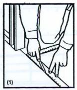
Locate the center-line of the structural column and scribe a line on the floor on both sides which extend further than the dia. of the column cover.
