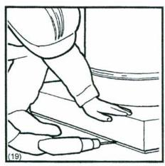
At caulk recess, fasten base assembly through to blocking.
