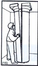
Locate mating column cover half and position around flange on other column half so as to insure proper fit.
