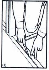
Locate center of structural column and scribe a line on both sides which extend further than the base to be installed later (step #18).
