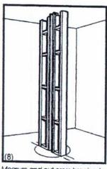
Measure and cut cross-bracing to appropriate lengths and instal @ 24" centers.
