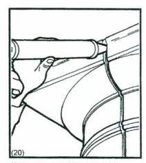
Using a low modulus, paintable caulking, caulk all seams including horizontal reveals at floor and ceiling.
