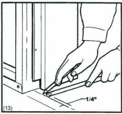
Place the column cover half with the outside diameter, 1/4" back of scribed center line.
