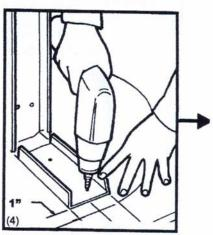
Fasten framing to structural column on center-line and plumb.
