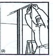
Use a plumb bob or laser to transfer center line onto ceiling.
