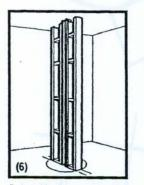
Cut and instal cross-bracing @ 24" centers.
