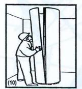
Locate mating half column cover and position around skeleton against vertical stud. Shim at base to match first column cover half.
