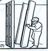
Locate first column cover half and position over scribed circular line on floor. Shim at floor if necessary.
