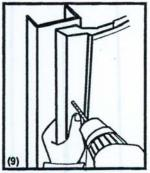
Drill pilot holes in center of flange on 16" centers starting at 5" from either end.
