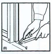
Place the half column cover with the outside diameter at the center-line.
