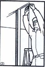
Use a plumb bob or laser to transfer center line onto ceiling.
