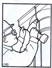
While ensuring that the column cover haves are held tight together use #10 x 1 1/4" "TEK" screws and fasten through both flanges into support stud down entire length of column covers.
