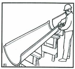
Measure length of column cover half from lower end to the point at which the diameter was measured in step #5. [Dim. "Y"],
