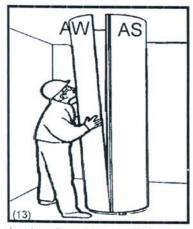
Locate mating column cover half and position around flange on other column half so as to insure proper fit.
