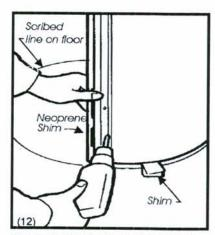
Shim bottom of column cover half until top is 1/8" from ceiling or passes through ceiling. Use neoprene shim between column cover and framing to insure O.D. of column cover is held. Plumb and fasten through previously drilled holes.
