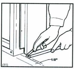
Place the column cover half with the outside diameter, 1/8" back of scribed center line.
