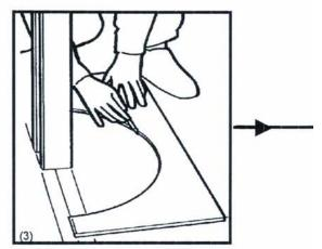
Cut "base" and "capital" plywood templates using paper outline supplied by DecoForm. Place "base" template on floor, center on structural column and trace entire outline. With "capital" template, duplicate this procedure on the ceiling tracing the rectangular profile only.
