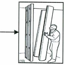
Locate column cover half as identified by the larger, Indented vertical flange and position over scribed circular line on floor.
