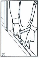
Locate center of structural column and scribe a line on both sides which extend further than the base to be installed later.
