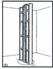
Measure and cut cross-bracing to appropriate lengths and instal @ 24" centers.
