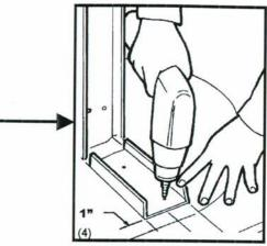
Fasten framing to structural column on center-line and plumb.
