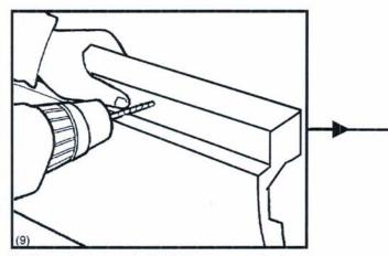
On the column cover half with the larger vertical flange ("AS"), drill and countersink hole 6" from lower end of column cover half and at 16" centers thereafter. Repeat on other column cover half starting at 5" from lower end but drill holes in center of flange as well as into the overlap joint at capital. Refer to drawing "A" (lower right of opposite page).
