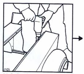
Into the "base" and "capital" caulk recess, drill 3/16" dia. clearance holes in caulk recess, 6" from each end.
