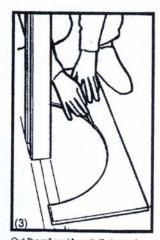
Cut "base" and "capital" plywood templates using paper outline supplied by DecoForm. Place "base" template on floor, center on structural column and trace entire outline, With "capital" template, duplicate this procedure on the ceiling tracing the rectangular profile only.
