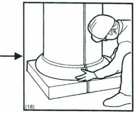
Position both base halves around column cover assembly. Fasten both base halves together through vertical reveals.
