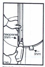
Shim bottom of column cover half until top is 1/8" from celling. Use neoprene shim between column cover and framing to insure O.D. of column cover is held. Plumb and tasten through previously drilled clearance holes.
