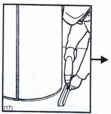
Position blocking along inside of both scribed lines and fasten to floor.
